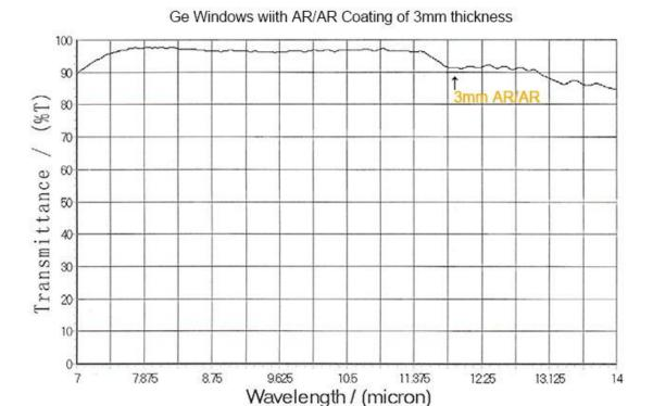
4. Transmission curve for Ge windows with coating AR/DLC of 3mm thickness
